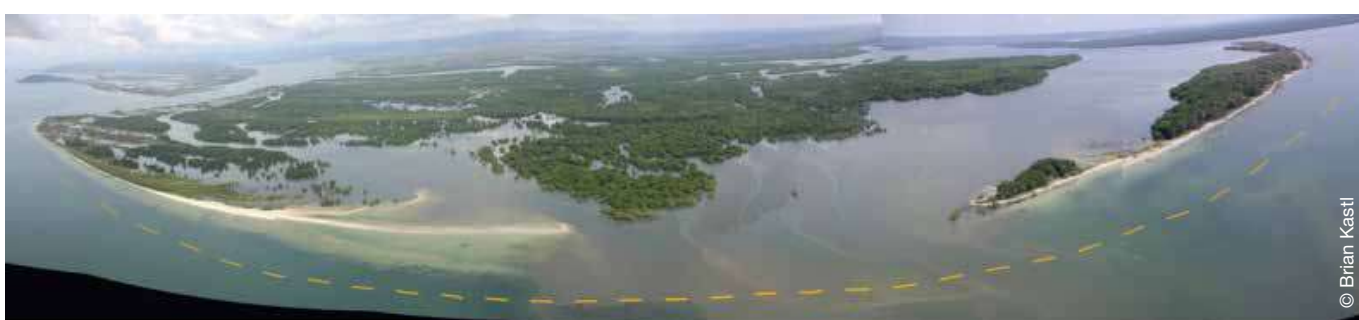
Figure 4: Aerial photograph of barrier beach captured 12 November 2012 by helicopter. The orange line represents the barrier beach location in 1994, during which time the beach was continuous without the current gap.
