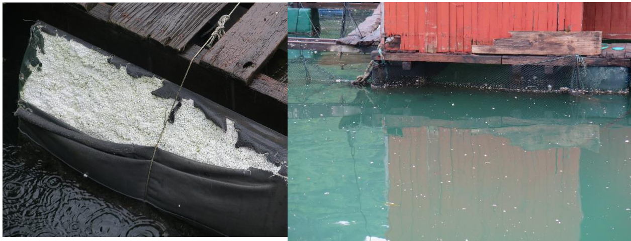
Photos: ripped canvas and small pieces of foam was released into the water© Pham Tuan Anh, 2016
