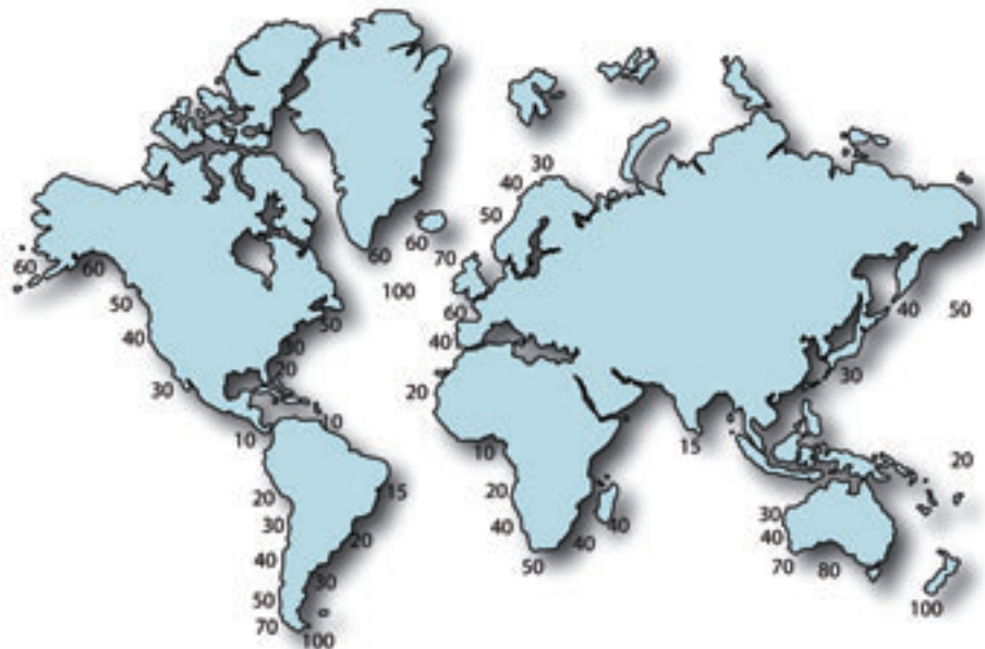
Figure A3-1: Wave power density (kW/m) of wave front in different parts of the world (Adapted from Langhamer, 2009b)
