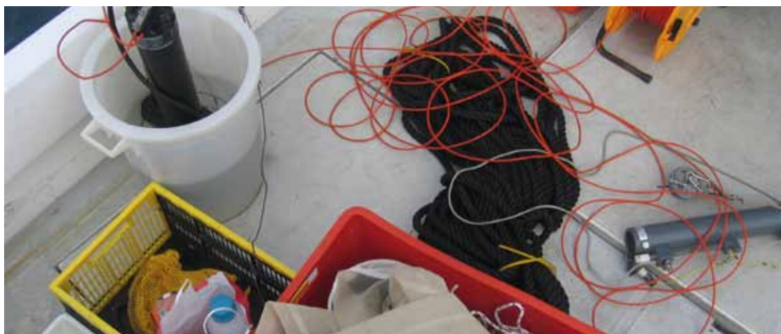
Multiparametric probe for measuring seawater quality. Photo: M. Tempesta
