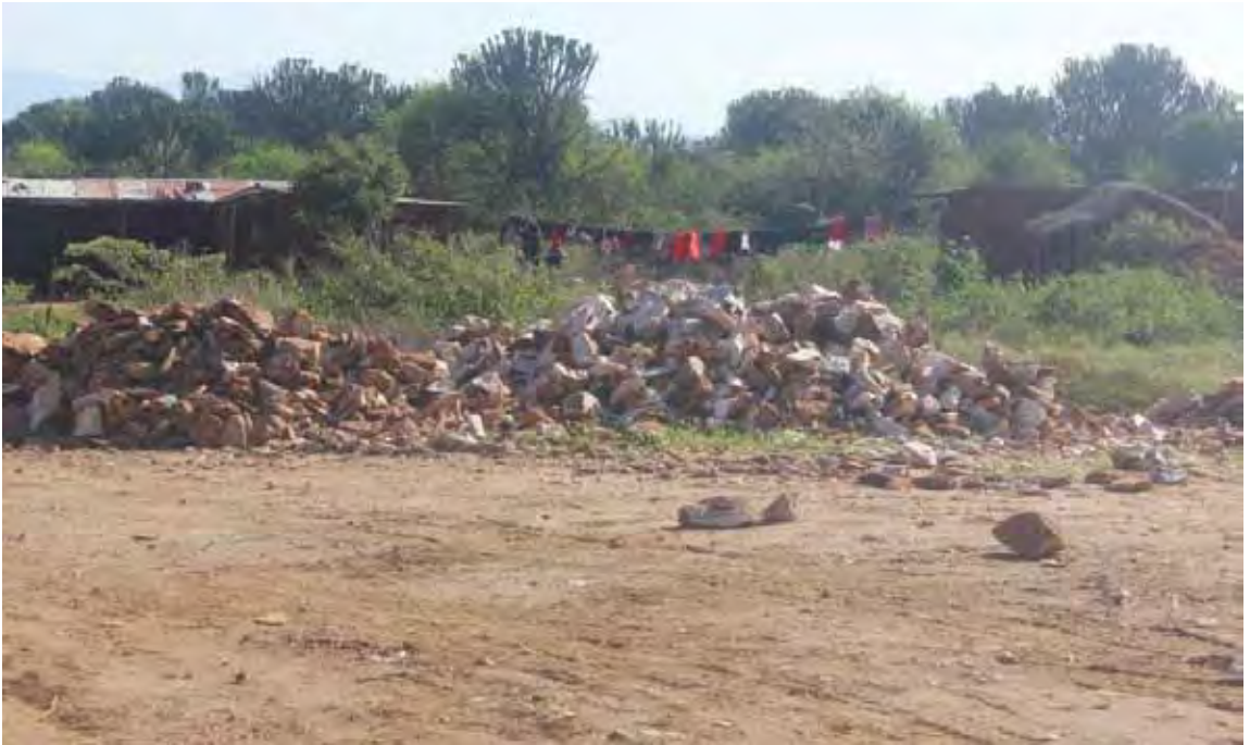
Piles of marble crushed by artisanal miners are ready to be loaded on trucks and used as limestone for cement production (photo 4.6).
