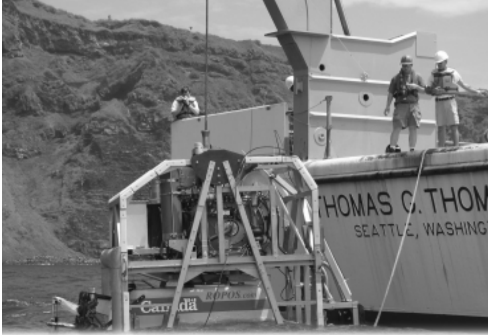
Launch of ROPOS remotely-operated submersible from the Research Vessel Thomas G. Thompson, at a hydrothermal vent site near the Maug Islands, in the Mariana Island Arc, South-west Pacific. Photo: Kim Juniper, University of Quebec at Montreal.
