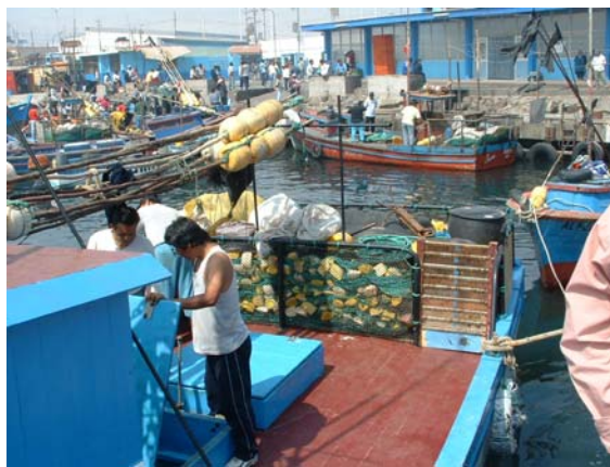
Fig. A6.8. Stored mainline in stern of fishing vessel. Note the mainline with integrated floats and the wood planks holding hooks to the right.
