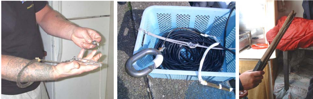
Fig. 6.1. Some of the tools used by longline fishermen to immobilize and retrieve terminal tackle from sharks. Hawaii longline fisherman demonstrating how he clips a loop of rope onto a branch line below the weighted swivel at the top of the wire leader to assist with removing a hook from caught sharks (left); ring and electrical cord of a “shocker” device used by a Japanese nearshore longline fishermen to immobilize sharks (middle); Chilean fisherman’s improvised dehooker (right) (photos by E. Gilman, J. Mangel, T. Miyamoto).
