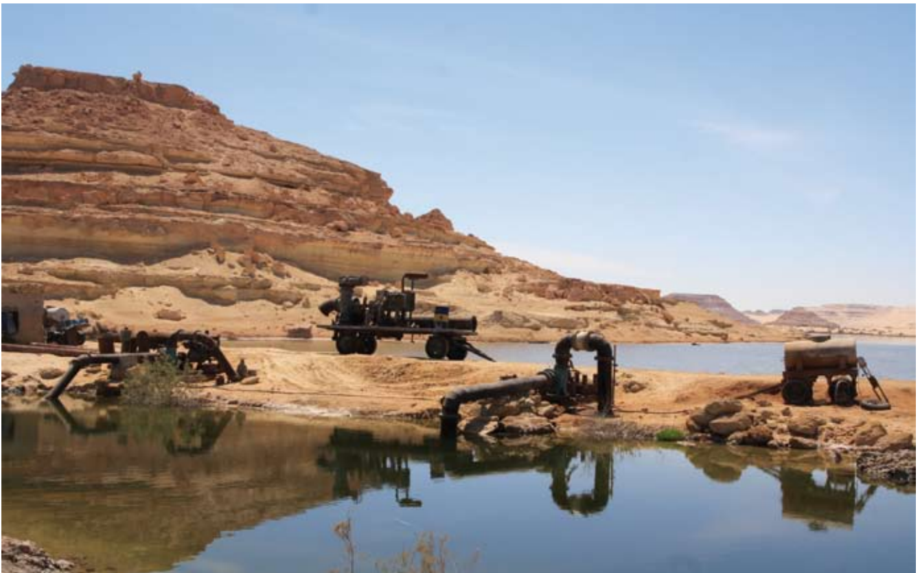
Pumps for water extraction in the Siwa basin, Egypt. Photo © Kevin Smith
